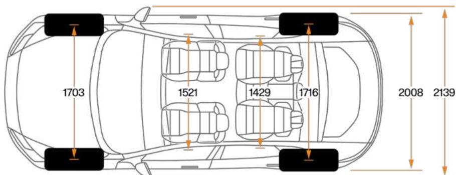
Abmessungen (mm): L-4840 mm H-1534 mm B-2139 mm
